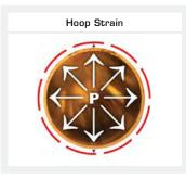
**DID YOU KNOW?** The only time copper tube will fluctuate in length (S<sup>1</sup>) is during expansion and contraction due to temperature. The only time copper tube will fluctuate in diameter (S<sup>2</sup>) is during expansion due to pressure.
